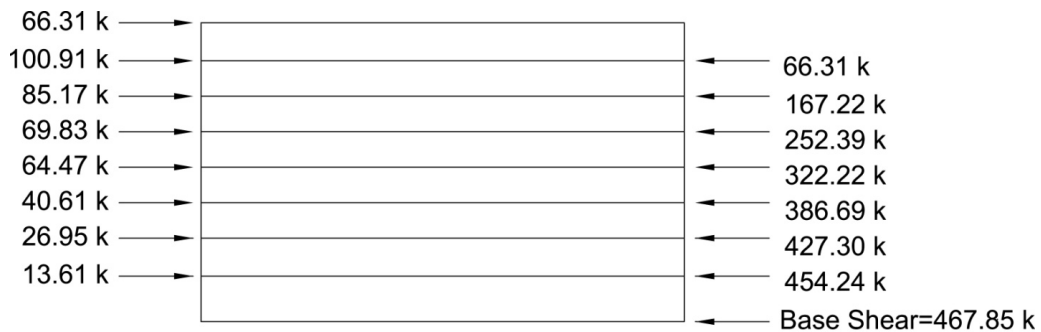
Figure 15: Diagram of Seismic Design Story Shear Forces
